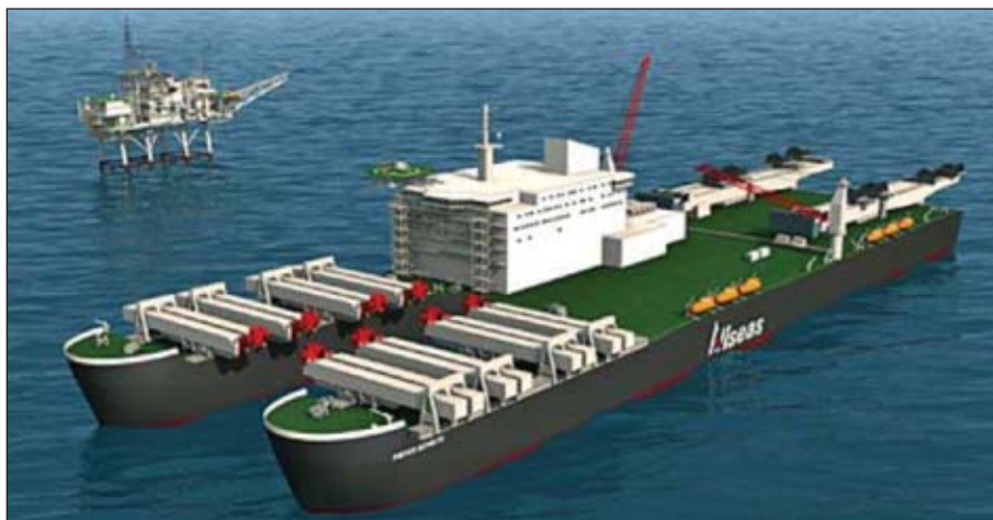
Allseas's Pieter Schelte platform installation-decommissioning and pipelay vessel (382 m long) will focus on global large-diameter pipeline installations and platform decommissioning in markets such as the North Sea once launched in 2013 (Photo: Allseas Group, Fig. 3).
