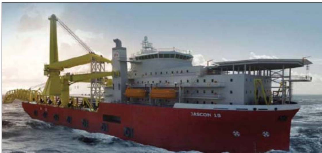
The 150-m Jascon 18 is a dynamically positioned ship-shaped pipelay and construction vessel capable of laying pipe up to 48-in. OD once it enters service in 2010 (Photo: Sea Trucks Group, Fig. 2).
